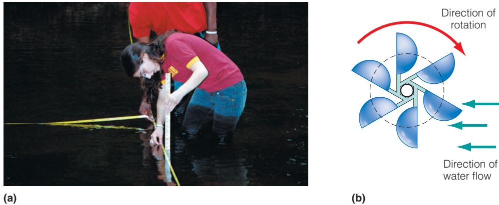
Figure 2 (a) Stream velocity can be easily measured using a cup-type flow meter. (b) As the water flows, the cups rotate about a fixed point on the instrument. The number of rotations per unit time provides an estimate of water velocity.
